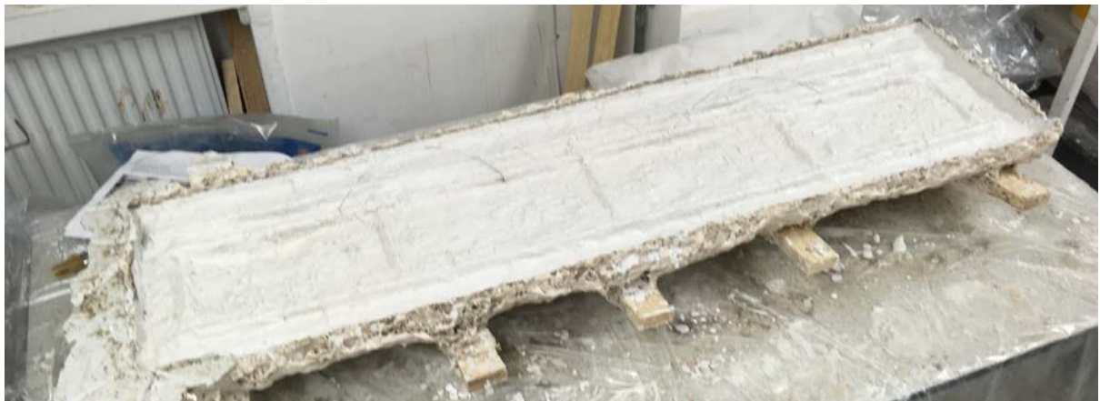
Ciment fondu brushed into mould Metal rods placed on back Metal rods secured with fibre-glass coated ciment fondu
