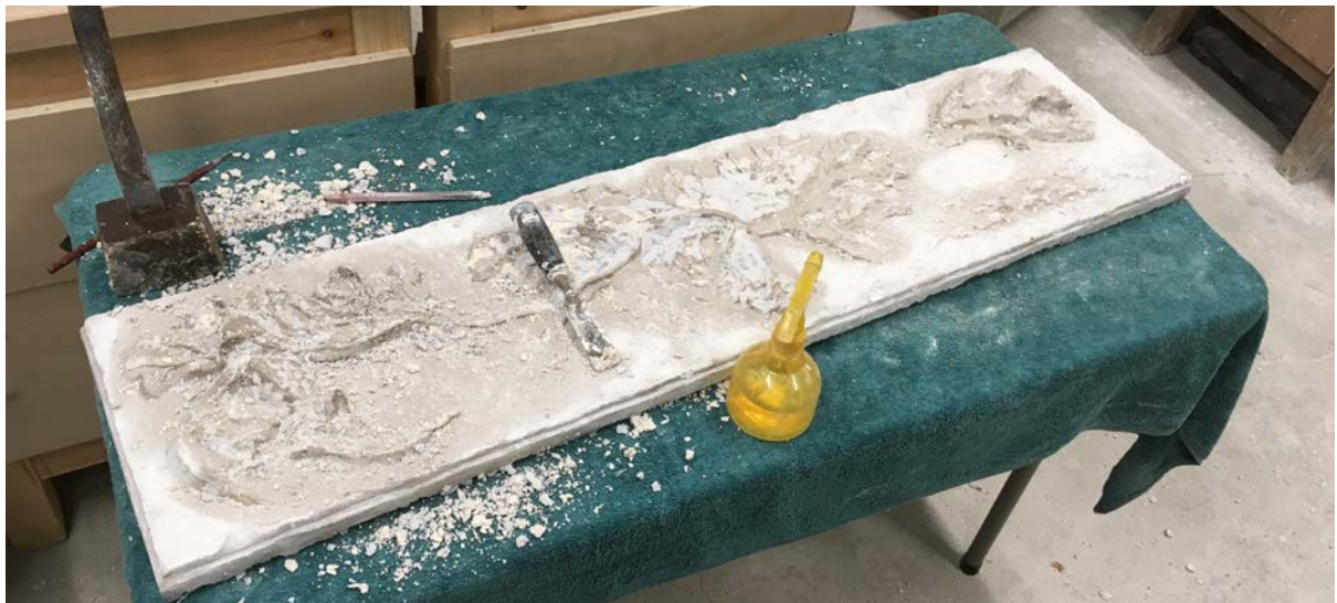
After ciment fondu has cured, mould turned over on wet towel Battens and plaster chipped off Careful removal of final pieces of plaster
