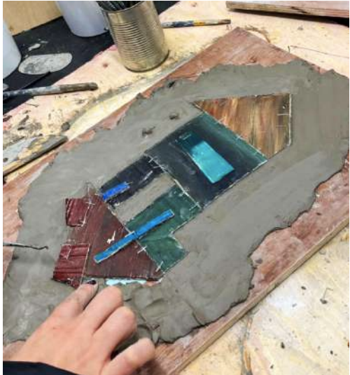
Silicone/ clay bed mould making process using cardboard sculpture
