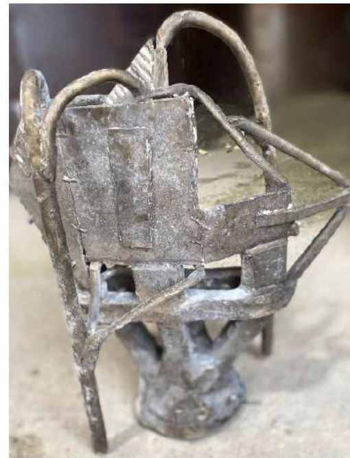
Wax mould of sculpture on wax cup with running systems added (image 1,2)- Bronze sculpture after pour ( Image 3)
