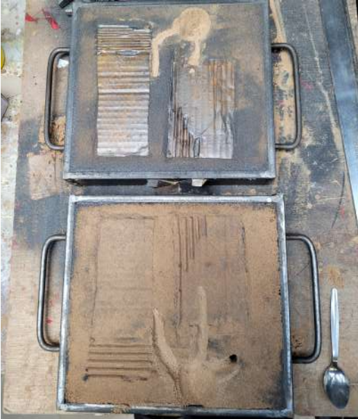
Sand casting tests/process with cardboard pieces
