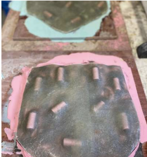
Silicone and fibreglass jacket with parts from cardboard sculpture
