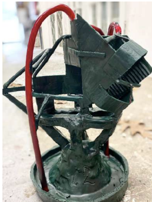
Wax mould of sculpture on wax cup with running systems added (image 1,2)- Bronze sculpture after pour ( Image 3)
