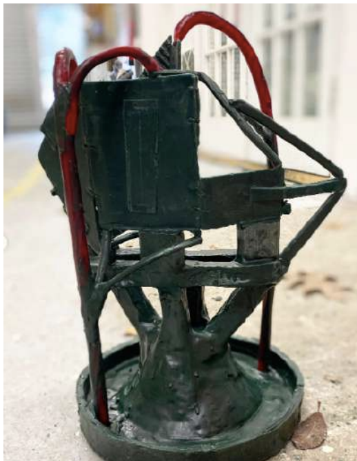
Wax mould of sculpture on wax cup with running systems added (image 1,2)- Bronze sculpture after pour ( Image 3)
