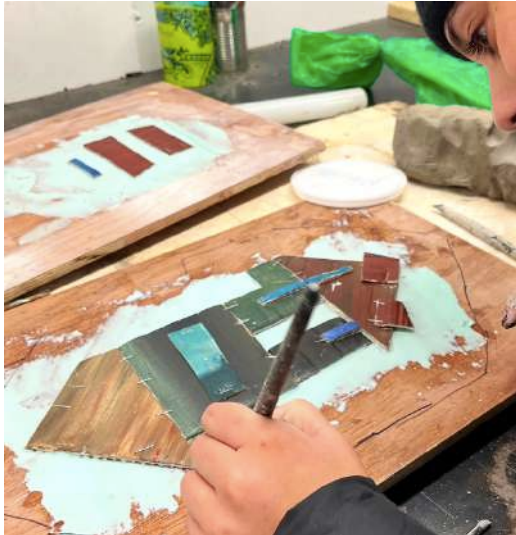
Silicone/ clay bed mould making process using cardboard sculpture
